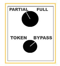
An example of the three position switching would be where either increased intensity light of different fields are being illuminated. The time per coin is varied 1/3, 2/3 of the full set time.
