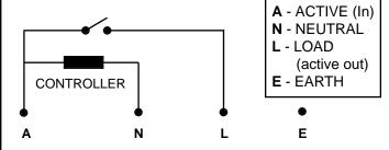
Supply voltage 240 Volts 50 cycles. Electronic units also available in 12 Volt operation.
